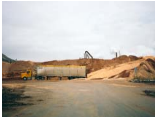
Figure 7. Live-floor van dumping on storage pile.
