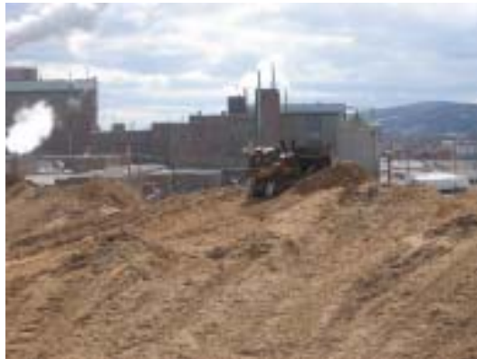
Figure 11. Crawler tractor pushing hog into mill infeed conveyor.
