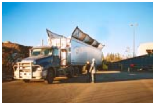
Figure 5. Live-floor trailer dumping onto a conveyor.
