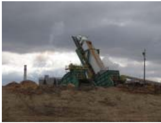
Figure 10. Unloading hog using a tipper.
