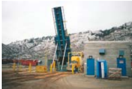
Figure 4. Side-by-side hog fuel tippers and B-train.
