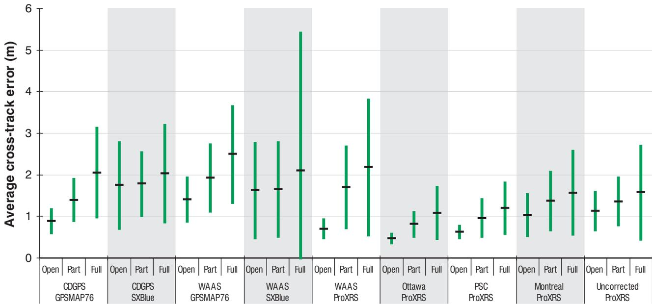
Figure 2. Means and standard deviations of average cross-track errors.
