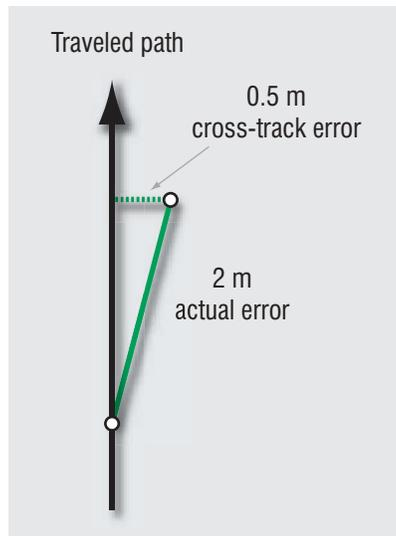
Figure 6: Example of actual and cross-track errors.
