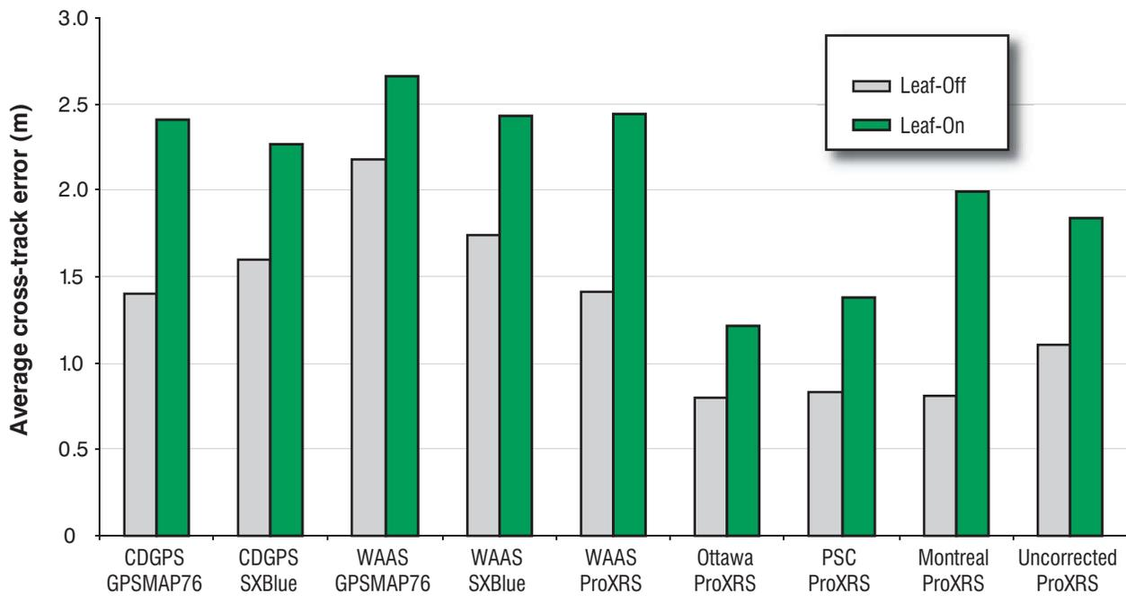
Figure 5: Average cross-track errors during leaf-on and leaf-off.
