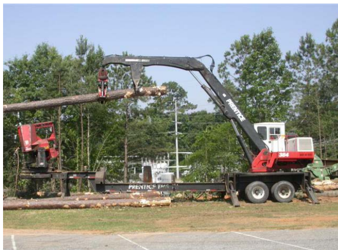
Figure 10: Trailer loaders include an integral delimber/topping saw for processing sawlogs. The loader also feeds the chipper.
