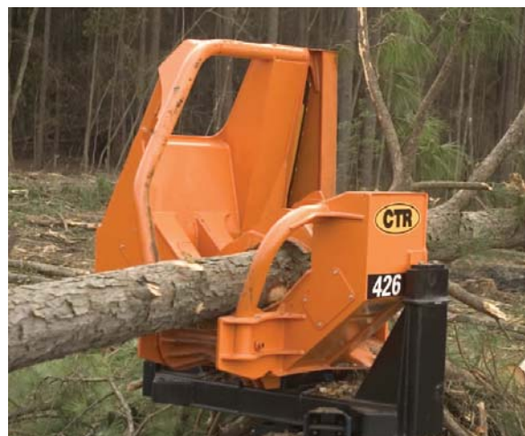
Figure 11: Pull-through delimber and cut-off saw can be paired with conventional loader for processing sawlogs.
