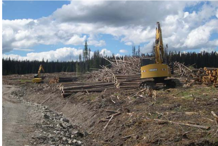
Figure 1: Two dangle-head processors working in tandem in a roadside logging operation.
