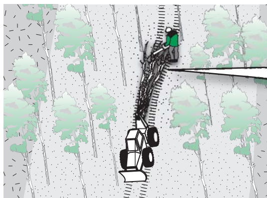
Figure 3. The various steps in a delimbing operation integrated with the extraction phase.
