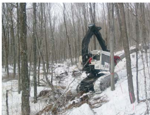
Figure 6. Maneuvering to place a felled stem near the edge of the extraction trail after felling in the secondary trail.
