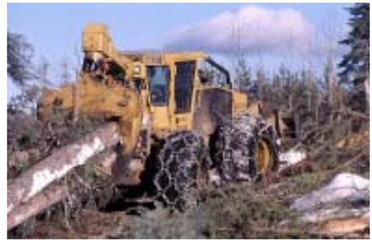
Figure 6. Tigercat 630B wheel grapple skidder.
