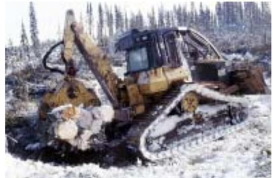
Figure 2. Caterpillar 527 track grapple skidder preparing bunches for the Caterpillar 545 wheel grapple skidder.
