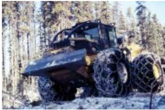
Figure 1. Caterpillar 535B wheel grapple skidder.
