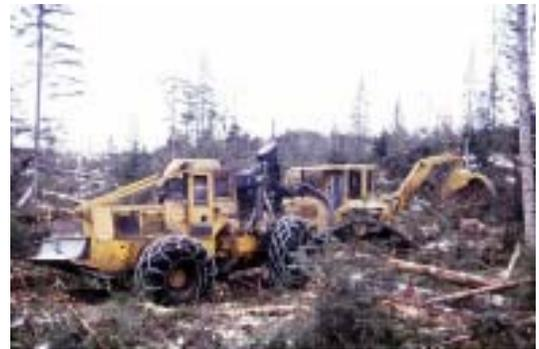
Figure 4. Caterpillar D5H TSK track grapple skidder preparing bunches for the Ranger F68G wheel grapple skidders.
