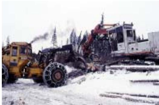
Figure 5. Link-Belt 3400 track loader decking stems skidded by the Ranger F68G wheel grapple skidders.
