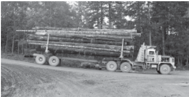
Figure 1. Loaded off-highway “fat” truck configuration.
