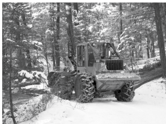
Figure 7. John Deere 540E line skidder.
