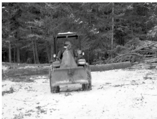
Figure 5. Ford tractor equipped with Farmi skidding winch.
