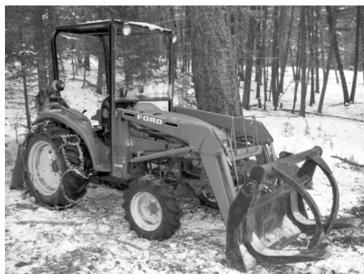
Figure 6. Ford tractor equipped with custom grapple.
