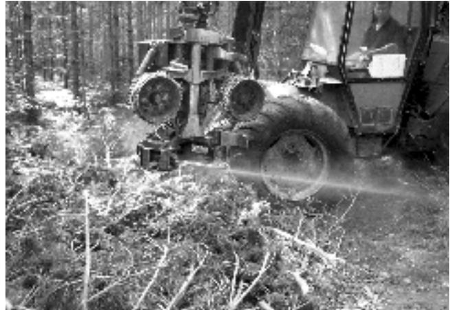
*Figure 2. The operator of a Valmet 701 harvester demonstrating the spray (white) produced by the Droppen R-500 sprayer.*
