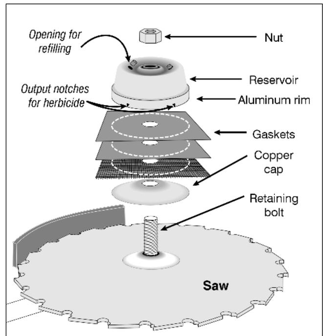
Figure 1. Schematic drawing of the Sprout-Less Herbicide Applicator.
