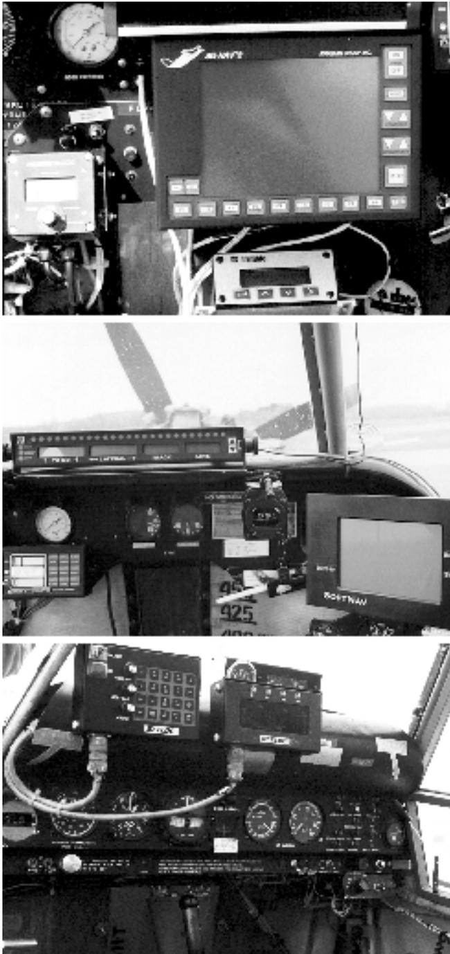
Figure 1. The Ag-Nav 2 (top), SoftNav (middle), and Satloc Air Star (bottom) GPS-based aerial navigation systems.
