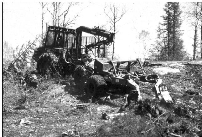
Figure 1. The Bräcke B290 patch scarifier mounted on a Timberjack 1010 forwarder.
