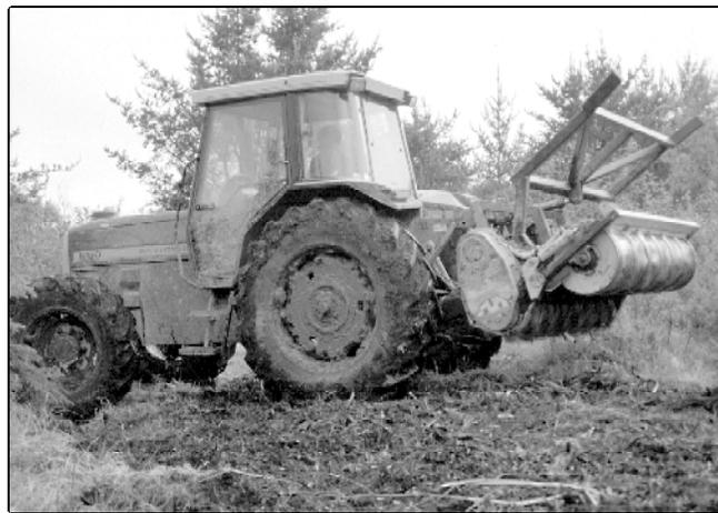
Figure 2. The Meri MJS-2.5 crusher mounted on the PTO of a Massey Ferguson 6180 tractor.
