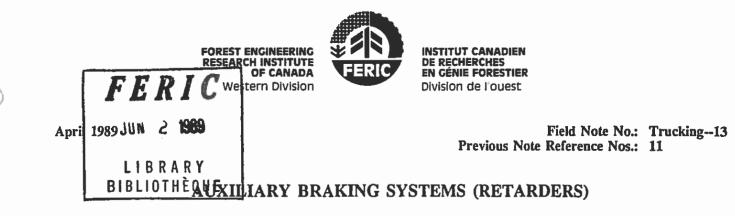
Auxiliary braking systems, or retarders, provide a means of slowing down a vehicle without using the service brakes. This contributes to vehicle safety by allowing the service brakes to remain cool and available in an emergency. Retarders also create the potential for reduced operating costs through less frequent brake maintenance and reduced tire wear.
