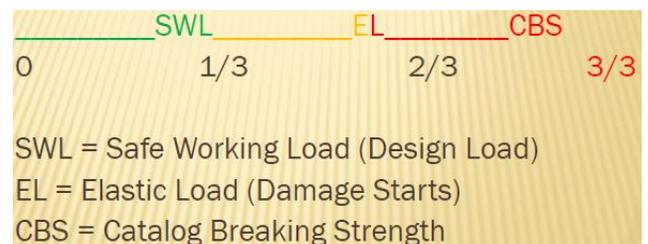
**Figure 7. Theoretical design loads of cables.**
