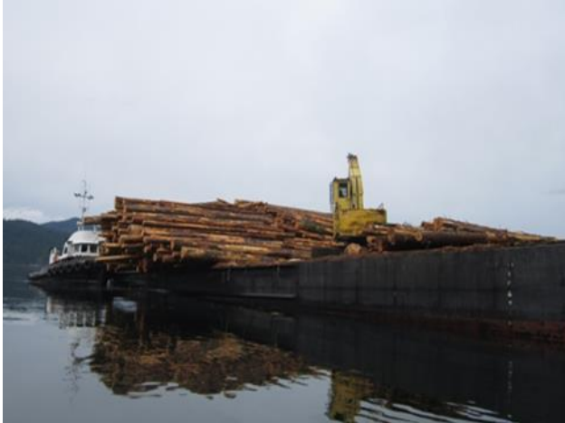
Figure 2. View of the barge being loaded by a log loader. Note the logs with much of their bark missing after being handled multiple times. Photo courtesy of BCTS.
