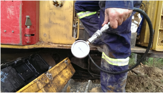
Figure 2. Hydraulic pressure gauge used for adjusting margin pressure and checking relief valve operation.
