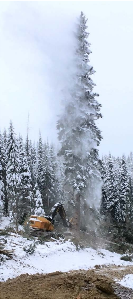
Figure 1. 2011 Tigercat 870C2 feller buncher cutting a large spruce tree.
