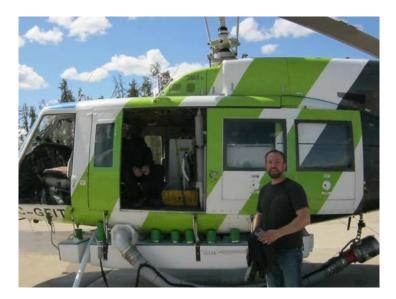
Figure 1. Isolair tank attached to a Bell 214B helicopter.
