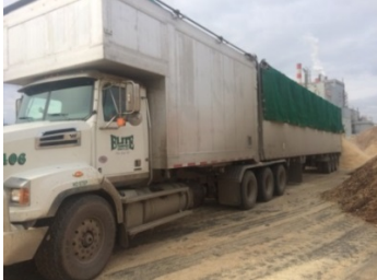
Figure 4. Elite Transport's auto-tarping system on its 7-axle chip trucks with walking floor.
