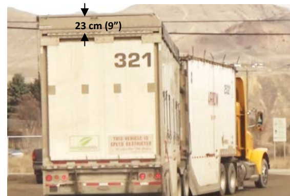
Figure 2. Test truck mounted with electrically operated tarping system on the rear trailer.
