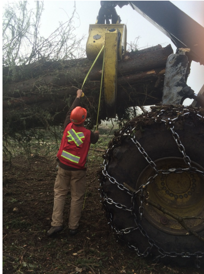
Figure 2. Measuring grapple height from ground to grapple pin, in this case the high position is being measured.
