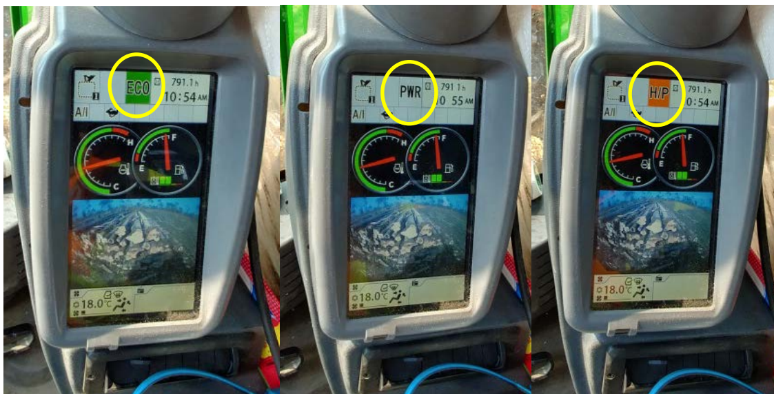
Figure 1. Operator-selectable power modes in this John Deere machine: ECO (economy), PWR (power), and H/P (high performance).
