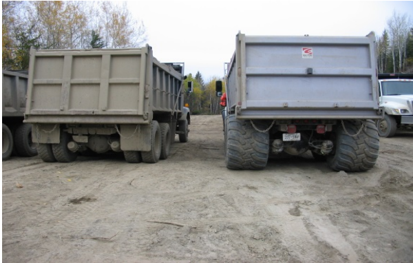
Figure 2. The use of tire pressure control systems (TPCS) and widebase tires can prolong road use and reduce impacts to the road surface.
