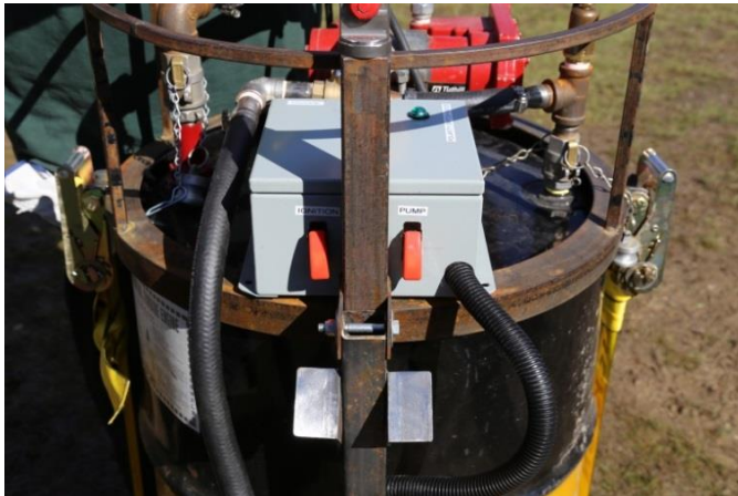
Figure 3. Switch realignment and polarity light addition.
