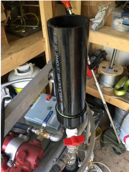
Figure 6. Mix funnel attached to an inlet port.
