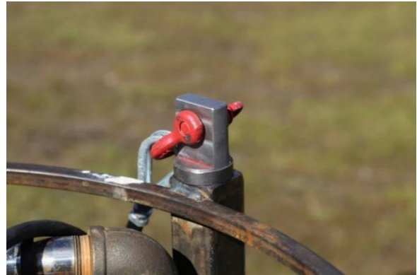
Figure 5. Custom turnbuckle attachment points.
