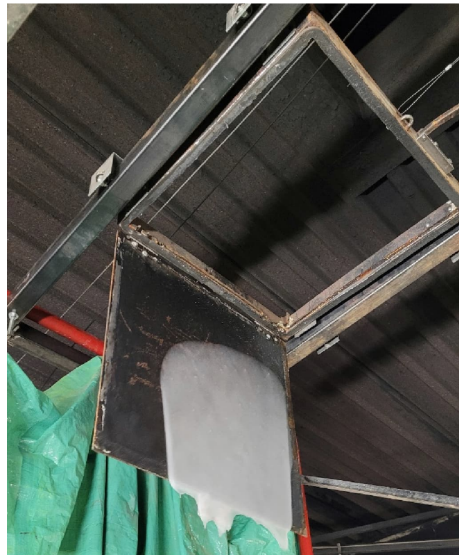
Figure 1. Barricade II at 2% mix ratio had a notable quantity of product stuck to the drop tank door.
