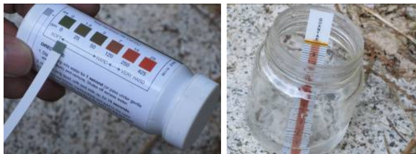
Figure 1. Test strips used to measure water properties have a colour reaction that is compared to a colour scale (photo on left shows total hardness reading); pH readings are collected in a similar manner. Titrator strips (right) are used for chloride readings. Test strips are inexpensive and available from www.HACH.com and www.CLEARTECH.ca .
