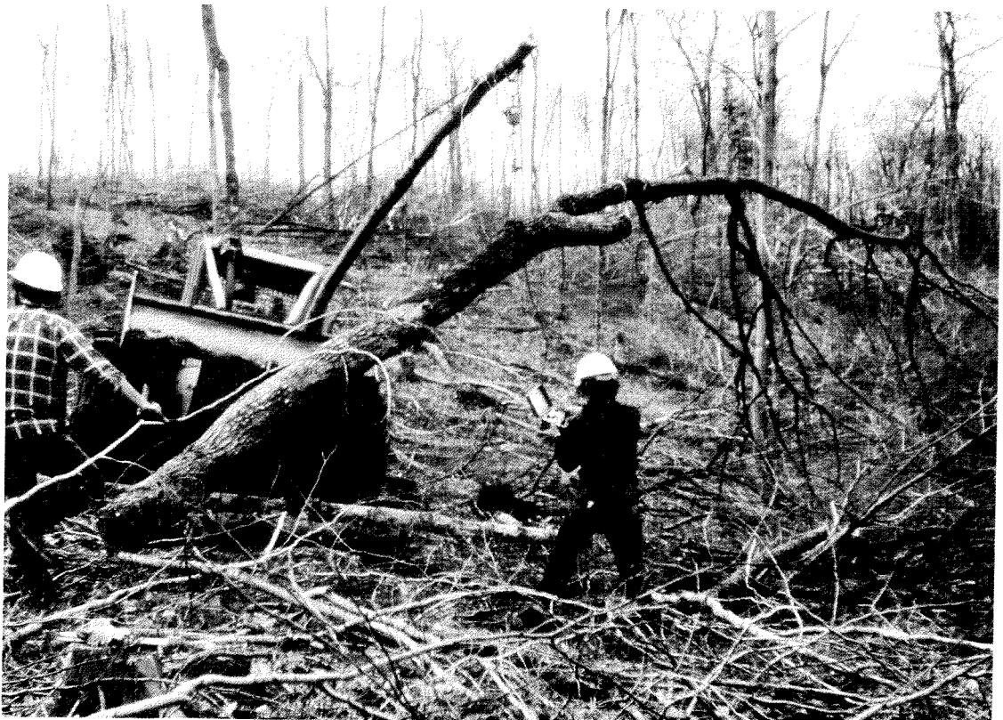
Photo no. 6: Tree-length sugar maple, Consolidated-Bathurst. Because of the logging method, the stand condition and the size of residue, a skidder was a great help in picking up tangled residue, weighing and clearing the plot.
