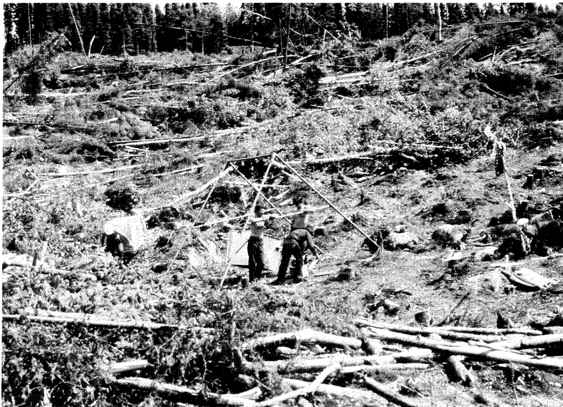
Photo no. 3: Shortwood black spruce, CIP. This is the balance frame and the containers used to weigh the residue. Note the difference between the plot cleared of all residue and the remainder outside the plot.
