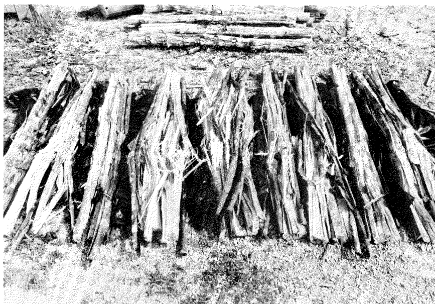
Figure 11. Yellow poplar bolts crushed with two pairs of rollers.
