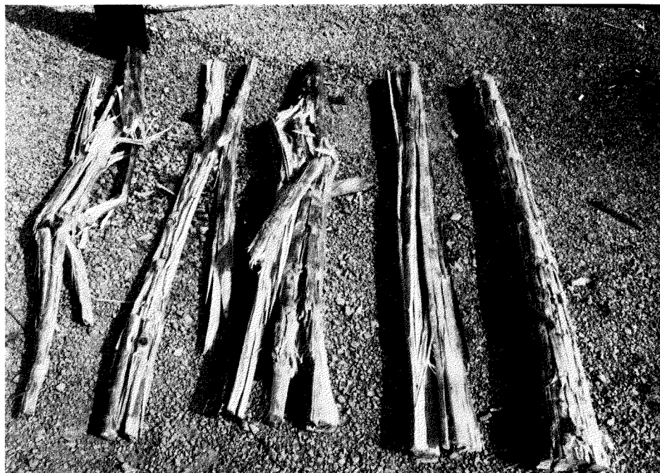
Figure 28. Effect of roller speeds on degree of fiberization.
