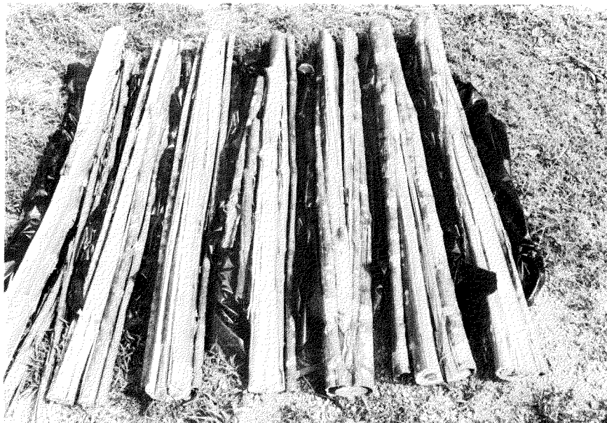
Figure 10. Yellow poplar bolts crushed with a single pair of rollers.
