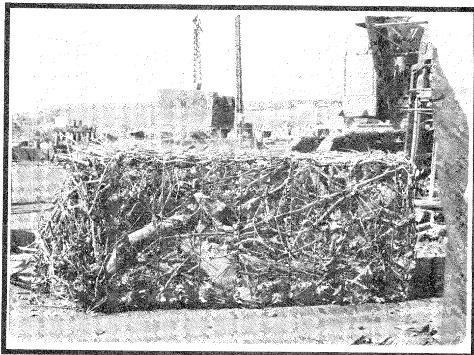
Figure 15. Scrub oak bale produced in paper baler. (Photo courtesy Harris Press Inc.)
