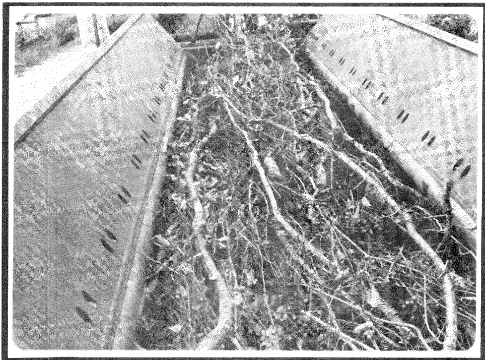
Figure 14. Scrub oak before baling in a folding box type portable scrap baler. (Photo courtesy Harris Press Inc.)
