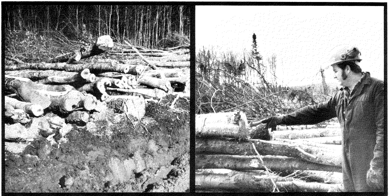
Fig. 6. Company B. Right - operator points to mud on logs resulting from skidding. Left - mud splashed on roadside piles by trucks.
