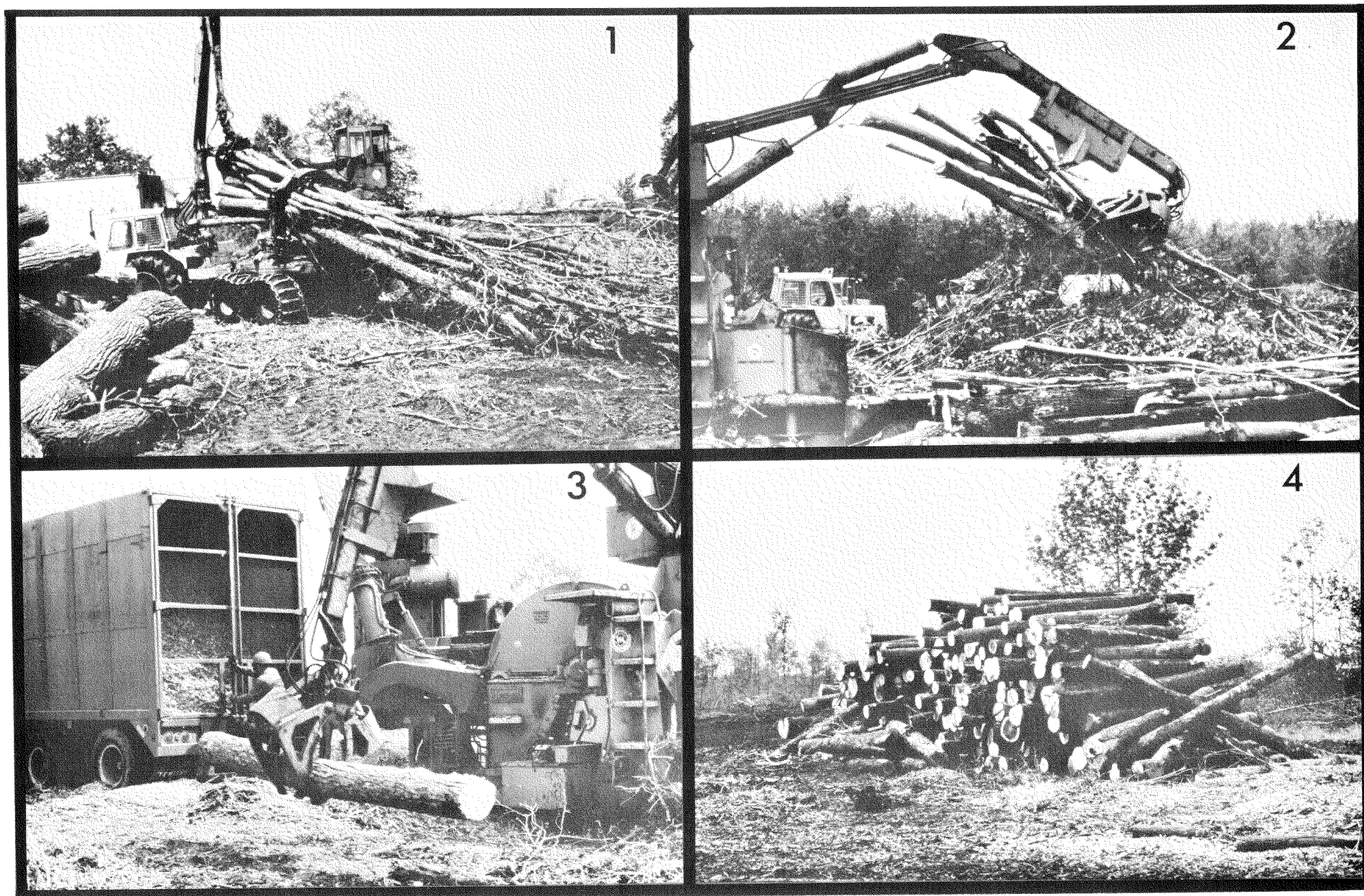
Fig. 3. Operating sequence at Company A: (1) whole-trees skidded by Volvo SM-868, (2) Chiparvestor loading whole-trees onto infeed conveyor, (3), (4) sawlogs separated and piled at the landing.
