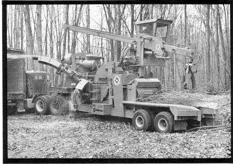
Fig. 8. Model 22 Chiparvestor with tractor unit attached, shown loading a chip van. The machine is equipped with a sliding boom loader and a dirt separator (debris chute). Photo supplied by Canadian Morbark Ltd.
