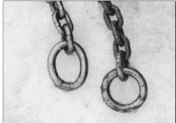
Figure 7. Deformed (left) and normal (right) sliding rings.
