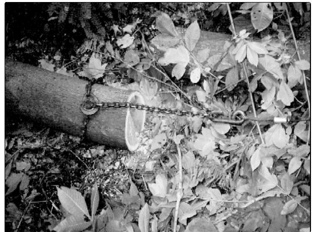
Figure 12. Chain choker (left) attached to mainline end hook (right).
