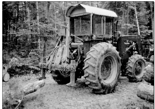
Figure 1. A tractor-mounted winch equipped with chain chokers.
