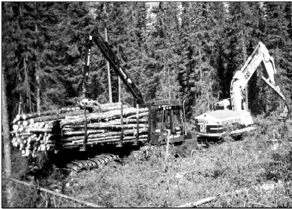
Figure 5. A Timberjack 1210 forwarder and a Caterpillar 320 harvester equipped with a Keto 150 harvesting head were used in the trials.
