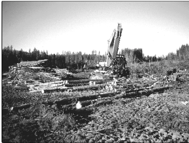
Figure 5. Multi-product processing with a single-grip processor.
