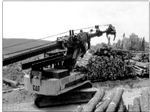
Figure 4. Sorting of products with a stroke delimber.
