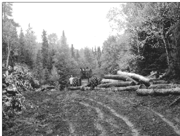
Figure 3. Unchoking stems into separate piles by species using a cable skidder.
