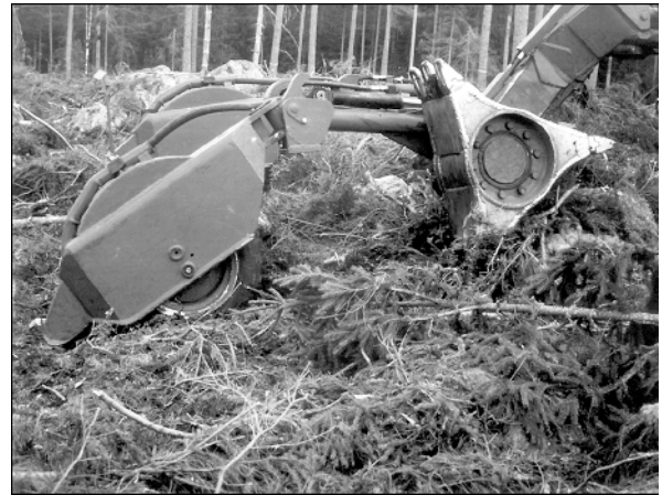
Figure 9. Soil-compaction wheels with seed-delivery tubes mounted behind a Bräcke B-290 mounder. (Photo credit: Anders Hildeman, SCA Skog)
