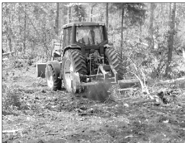
Figure 2. Mulching with the Meri Crusher MJ-2.3 mounted on a John Deere 6400 tractor.
