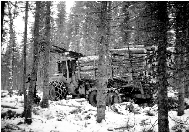
Figure 3. The Fabtek 546B shortwood forwarder.
