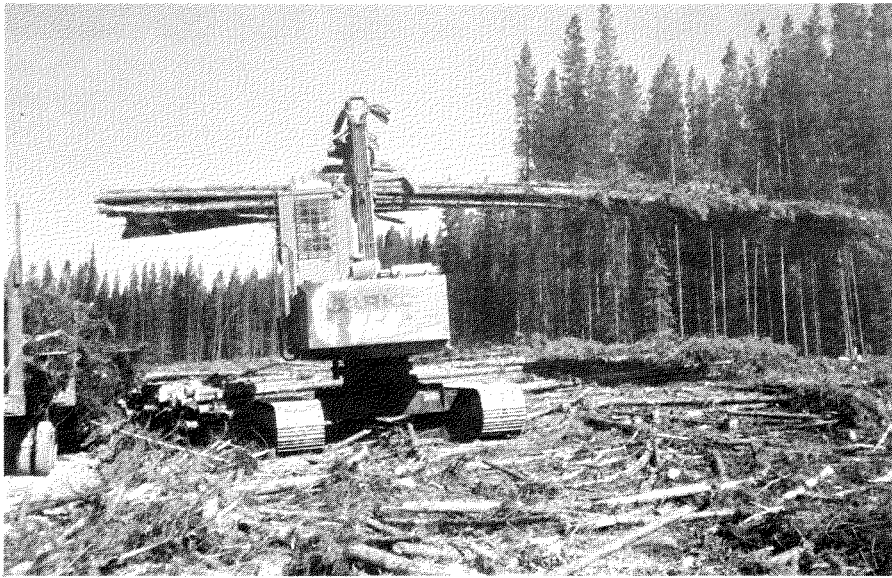
FIGURE C. Loading small pine logs from roadside piles on the skidder operation. Loader is working on a level site beside the road. The elevated position gives good visibility for loading off-highway trucks.
