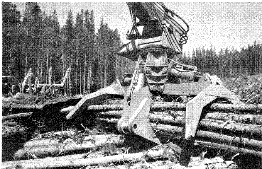
FIGURE B. Close-up view of grapple. Note the chain drive for 360° grapple rotation and the two hydraulic live heels.
