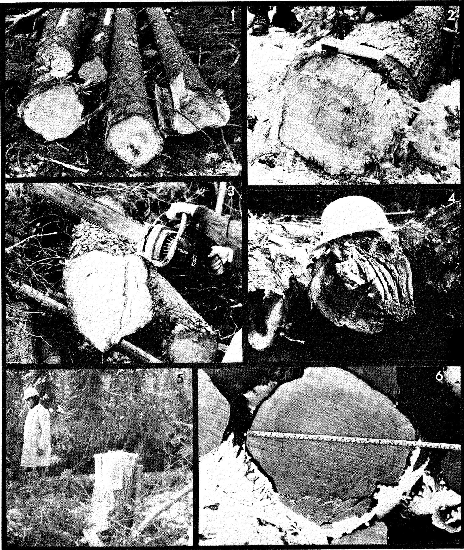
Figure 1. Wood damage from various felling machines, 1: Cat 950 harvester, Thunder Bay, Ont., June 1975; 2: QM Tractor-mounted shear, Okanagan Falls, B.C., Feb. 1977; 3: Earl's Para Shear feller buncher (F.B.), Okanagan Falls, B.C., March, 1977; 4: Drott 40 F.B., Dryden, Ont., Feb. 1978; 5: Repeated shearing attempts are evident on this stump, Drott 40 F.B. Timmins, Ont., Jan. 1977, Kockums 880 with chainsaw felling head, Prince George, B.C., March 1977.
