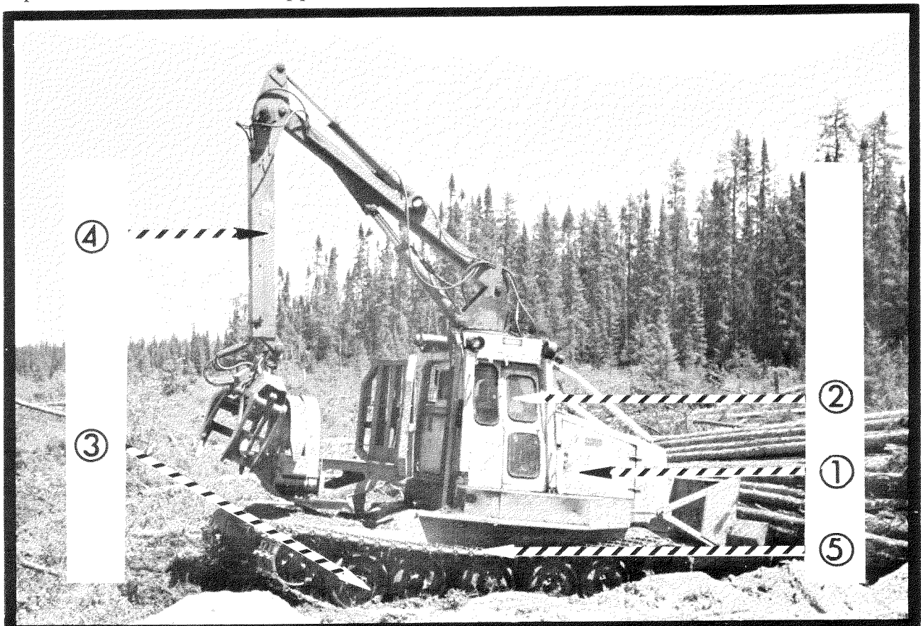
Fig. 3. The FMC Grapple Skidder
