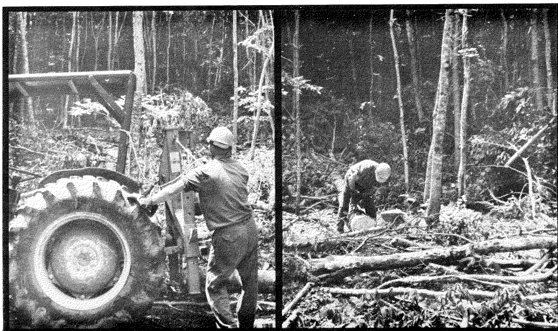
Fig. 4. Left — Operator is winching in a tree. Right — Operator attaches a chain choker.
