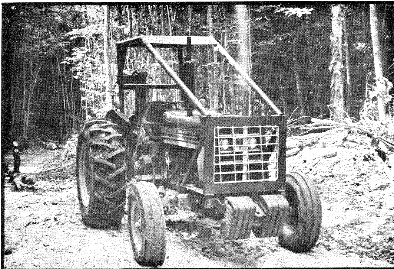
Fig. 3. Oblique view of tractor, showing modifications required for logging. The steel bar holding the weights requires bracing. The iron lattice in front of the radiator is too open for good protection.
