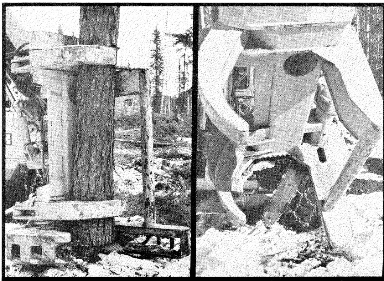
Fig. 6. The Kockums 880 saw attachment can fell trees up to 23 in (58 cm).
