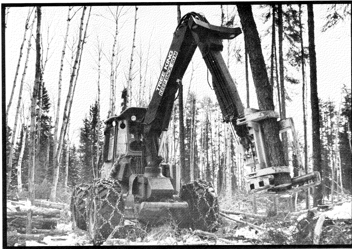
Fig. 7. The Kockums 880 equipped with standard tires and tire chains. Note the low-profile lugs on these tires.
