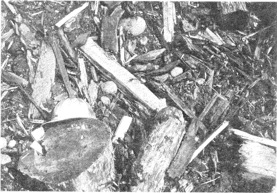
Typical log-sort yard debris: bark, broken wood and rock mixed due to mechanical log handling. (Piece size indicated by hard hat.)
