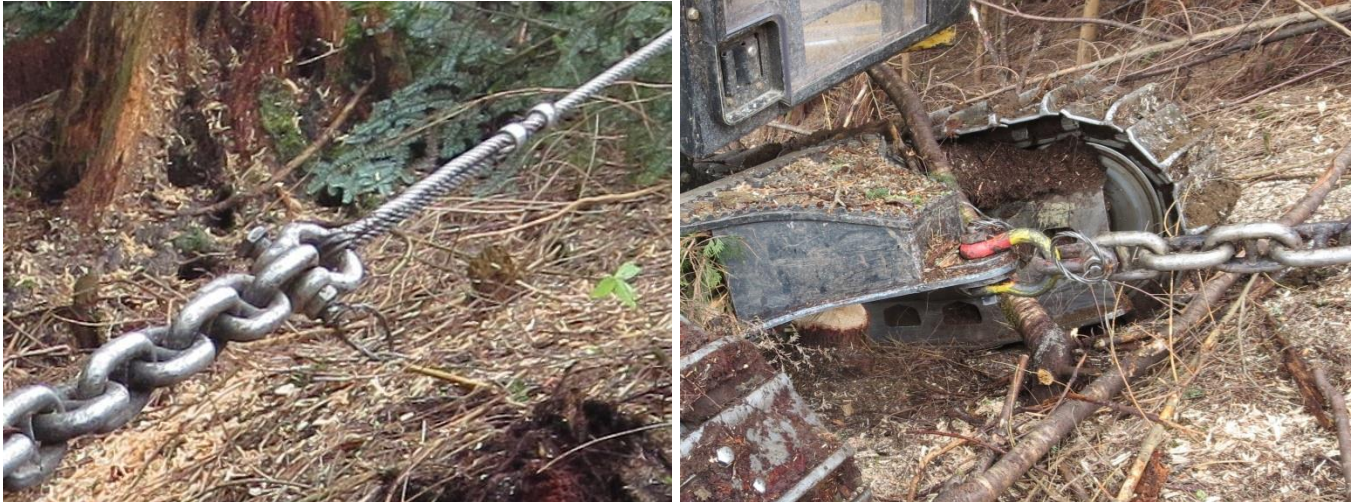
Figure 8. Swaged cable attached to a 4-m-long chain shackled to the feller-buncher.
