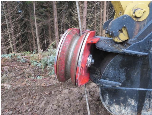
Figure 6. Boman fairlead sheave mounted on the bucket of the anchor machine.
