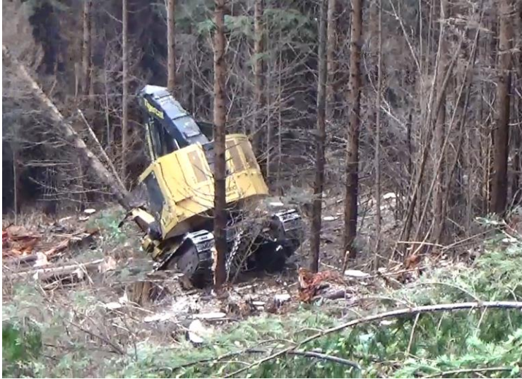
Figure 10. Feller-buncher with tracks rocking off the ground.
