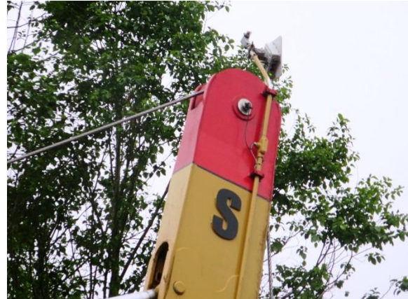
Figure 5. Sheave mounted on the anchor machine's stick extension.
