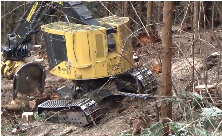
Figure 2. Tigercat LX830 C feller-buncher equipped with a Tigercat 5702 continuous-rotation disc saw, working below the road on a ~40% slope.
