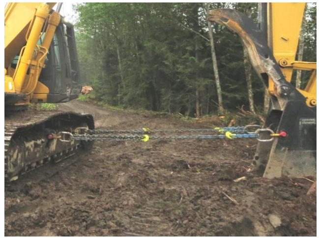
Figure 7. Chains securing the bucket to the anchor machine's track frame.
