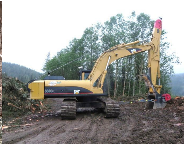
Figure 3. Caterpillar 330C L anchor machine positioned on the road above the harvesting area.
