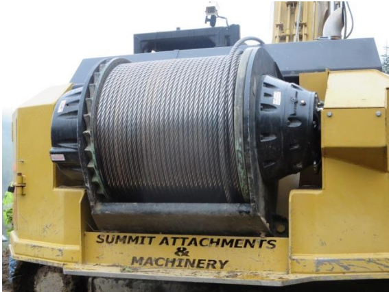
Figure 4. Winch mounted on the anchor machine's counterweight.
