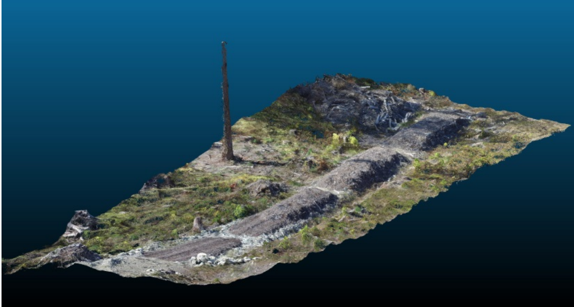
Figure 3. 3D model showing four debris piles along spur 2. Note the thin depth of debris within the first pile (far left), and half of the second pile, as well as the tall height and rounded top of the third and fourth piles. Also, the 3D model does not show live limbs on the tree because the data collection captured only the lower portion of the tree.
