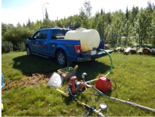
Figure 12. Pressure-testing equipment and set-up.
