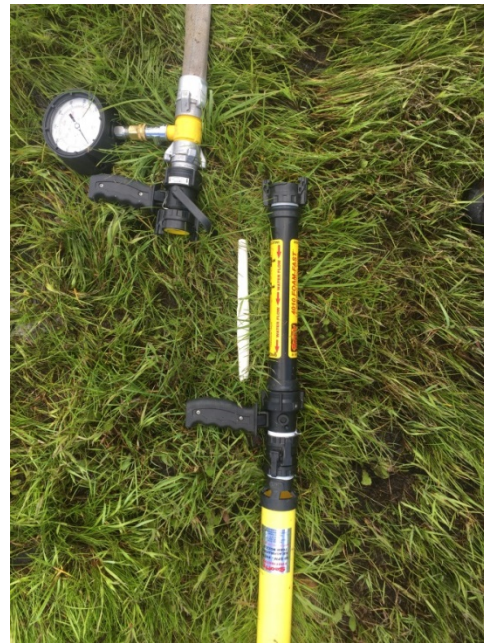
Figure 21. Foam stick deformity.
