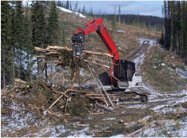
Figure 5. Construction of piles or windrows by excavator after harvest (photo by D Gossoo)
