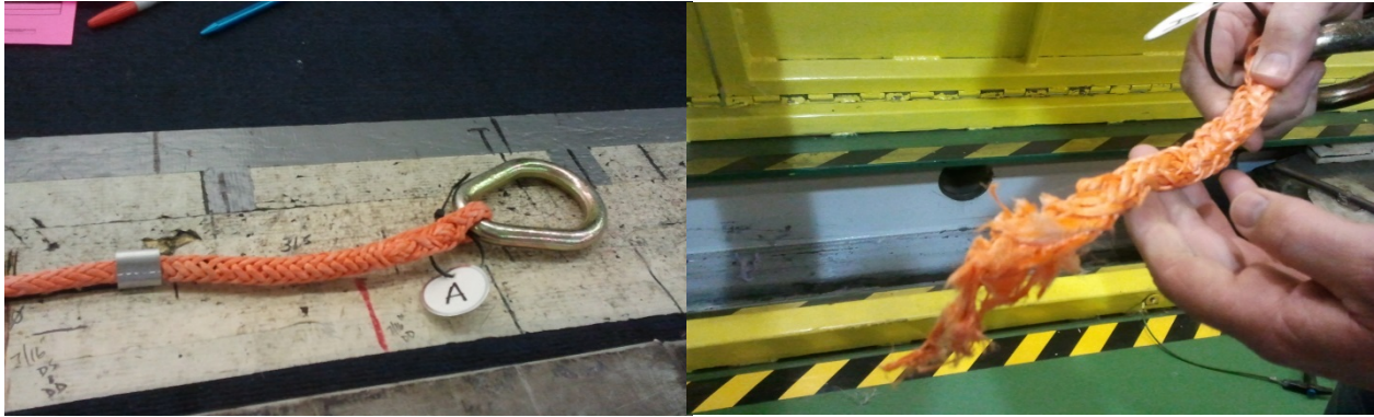
Figure 1. Sample A before (left) and after (right) break test.
