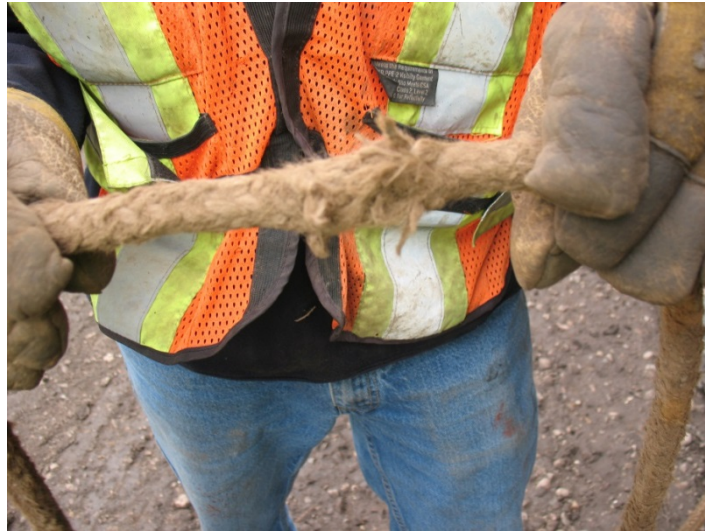
Figure 3. Rope with severed strands that is no longer suitable for service.
