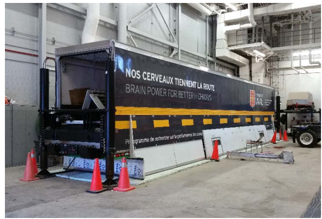
Figure 4. Heavy vehicle simulator in freezing mode, with insulation panels positioned.
