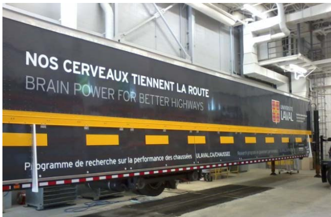
Figure 3. Heavy vehicle simulator installed above the test pavement.
