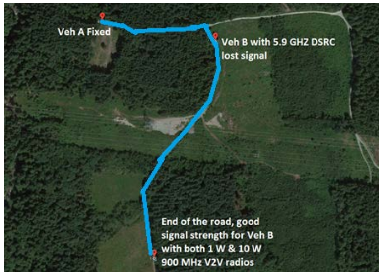
Figure 9. Comparison of 5.9 GHz and 900 MHz V2V communication range for measurement location 6.
