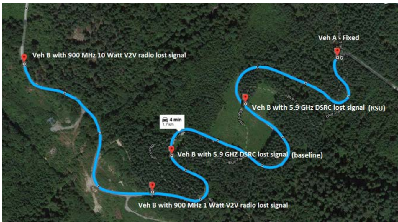
Figure 8. Comparison of 5.9 GHz and 900 MHz V2V communication range for measurement location 3.
