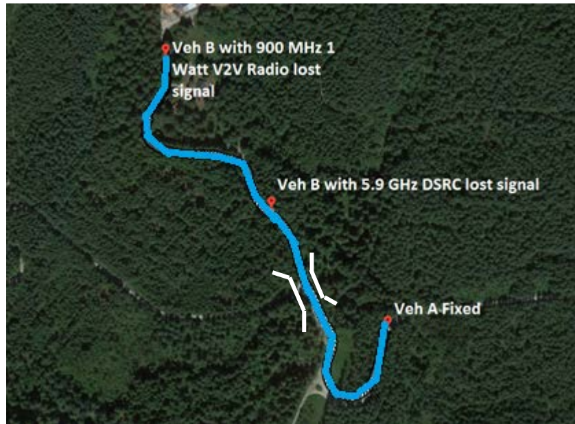
Figure 7. Comparison of 5.9 GHz and 900 MHz V2V communication range for measurement location 1.
