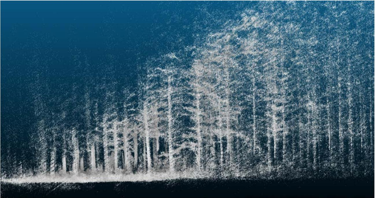
**Figure 8. Profile view (perpendicular to the scan line) of the point cloud from the +35 degree scanning angle.**
