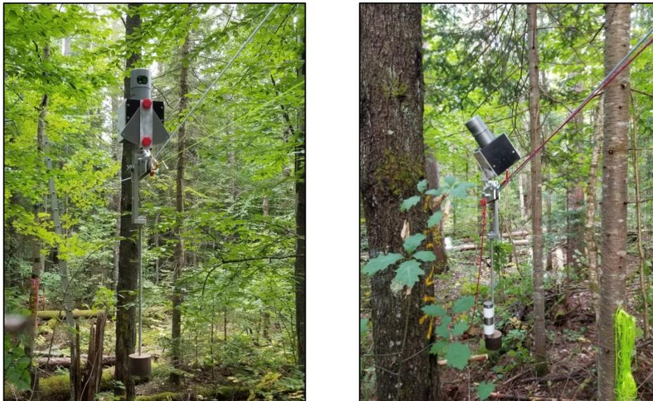
Figure 1. Mobile LiDAR system setup with 0° and 35° scan angles
