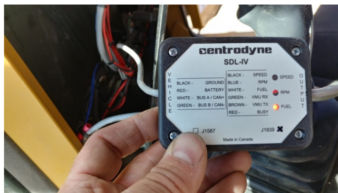
Figure 2. J1939 SDL module installation in a grapple skidder.
