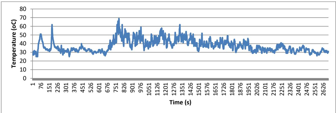
**Figure 7.** Temperature data collected at point 3. Temperatures were above 40°C for over 21 minutes.
